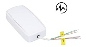
Efento 4-20 mA / 0-10 V sensor interface allows users to connect any type of analog sensor. Device can be equipped with up to four analog interfaces (2 x 4-20 mA and 2 x 0-10 V). Sensors can be powered either from the device's battery or by an external power source. Data from the analog sensors is presented as current (4-20 mA) or voltage (0-10 V).
